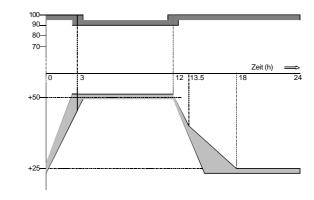
Fig.9 Load cells certified to OIML R-60 are tested to withstand 12 damp heat cycles.
